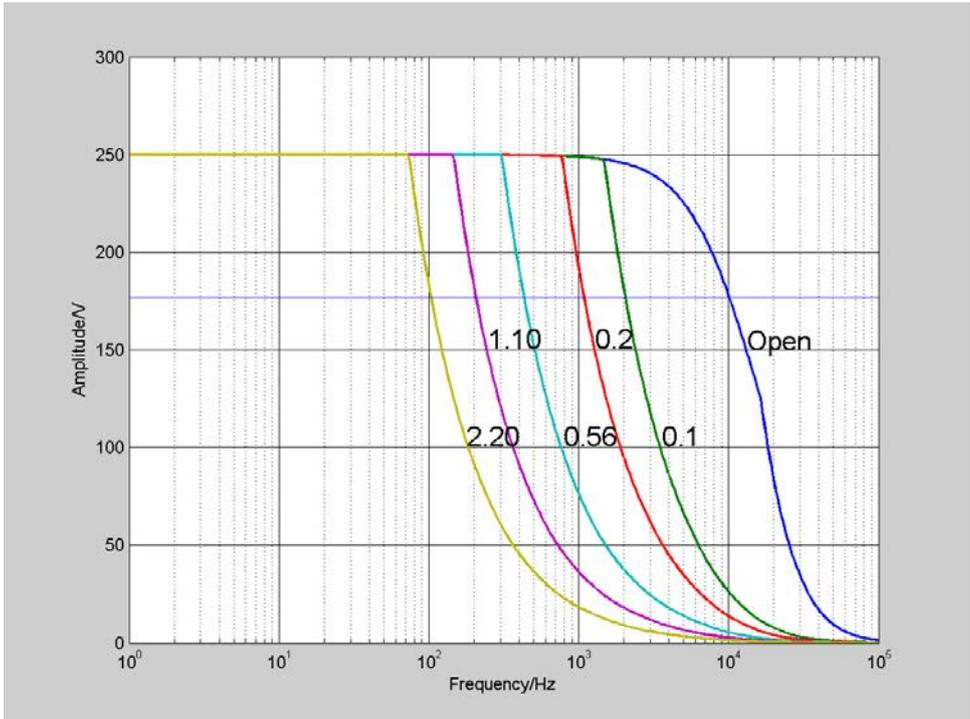
E-536.3x: Operating limits with various piezo loads, capacitance values in  $\mu\text{F}$
