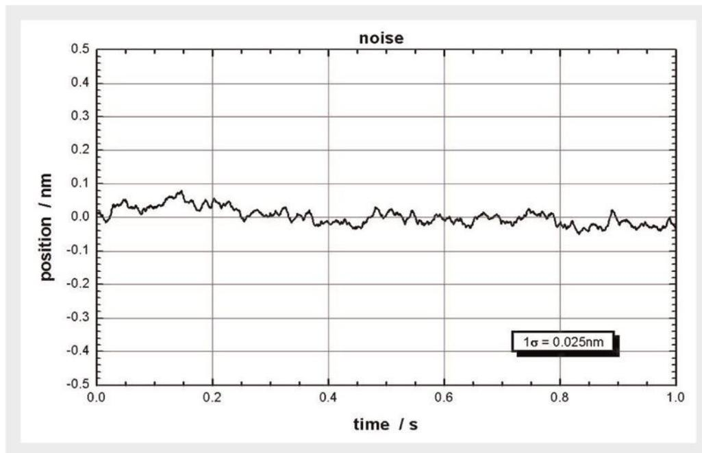
*The position measured by an ultrahigh-resolution external capacitive sensor shows that the resolution of the P-363 is under 0.05 nm with an E-536.3x (open loop)*
