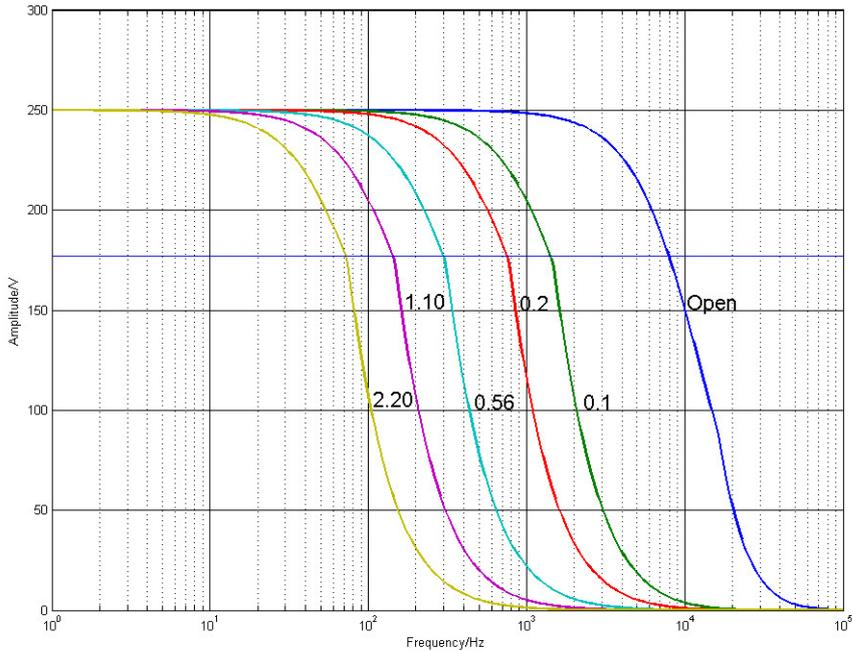
E-536.3xH: Operating limits with various piezo loads, capacitance values in  $\mu\text{F}$
