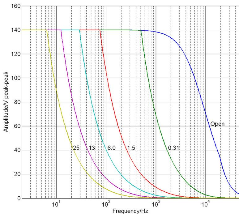
*E-625: Operating limits (open loop) with various piezo loads, capacitance values in μF*
