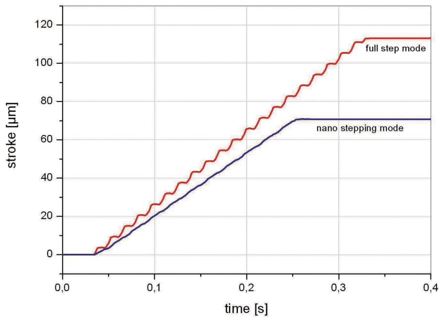
*Comparison of the motion type of a NEXLINE® actuator: The nanostepping mode provides very smooth motion. Full step mode allows higher speed.*
