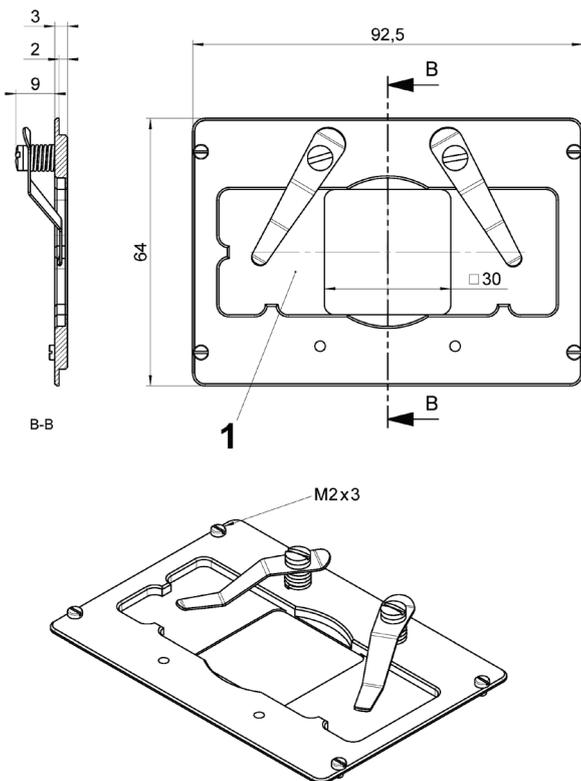
Accessories: P-545.SH3, microscope slide holder, dimensions in mm
