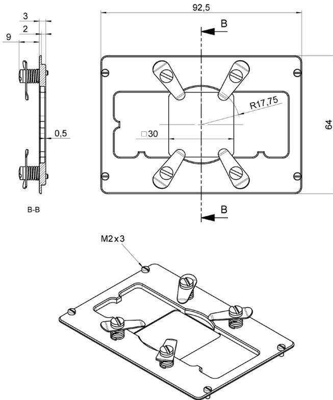
Accessories: P-545.PD3, Petri dish holder, dimensions in mm
