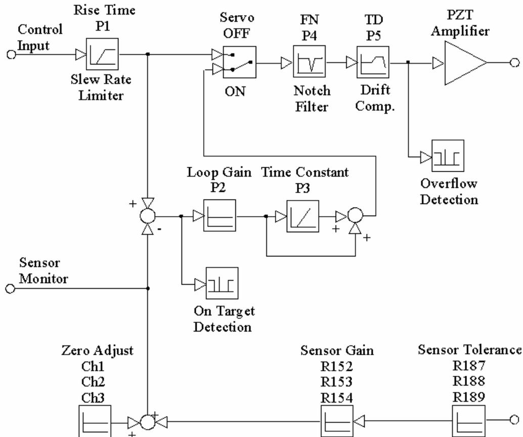
Fig. 2 E-664 block diagram
