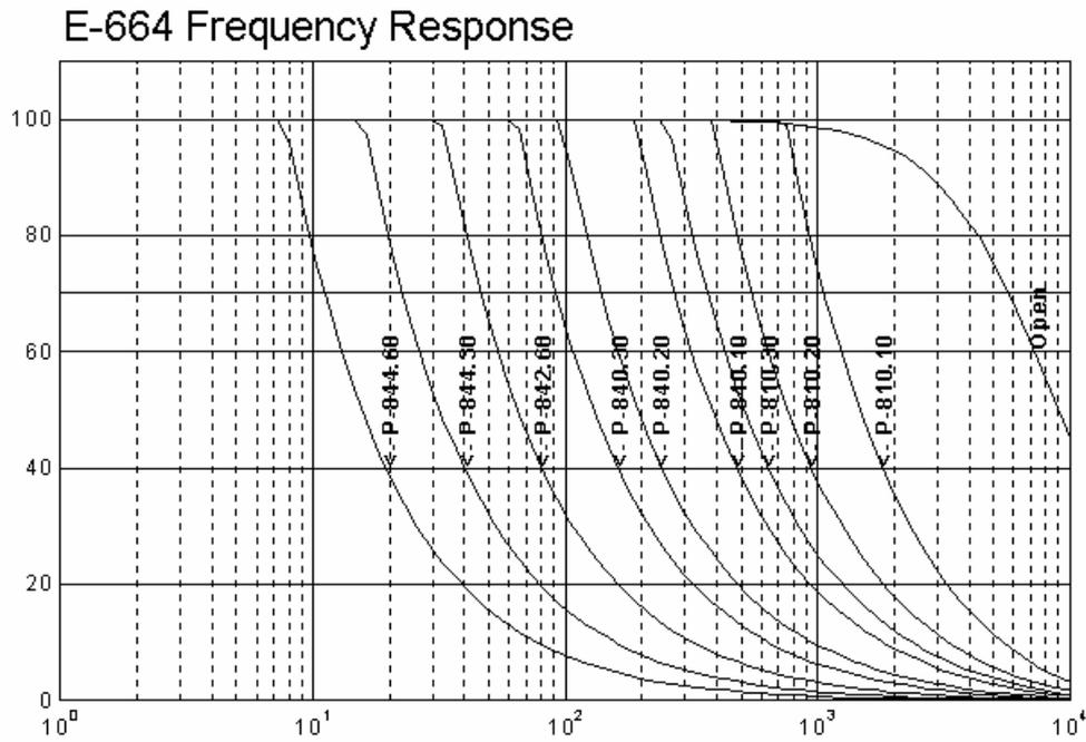
Fig. 4. Frequency response with a selection of PI PZTs
