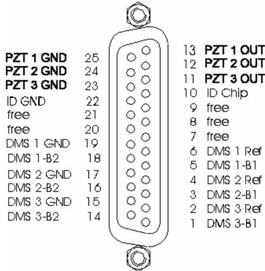
Fig. 7. Type: Sub-D 25 pin female
