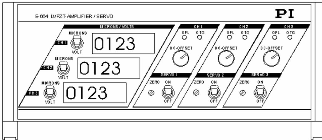
Fig. 5. Front panel operating and display elements
