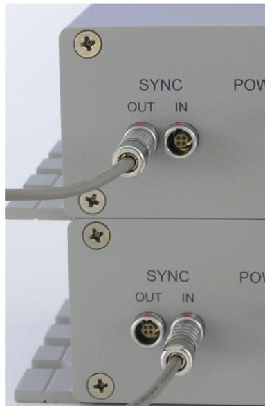
Fig. 13: Two E-852.10s connected with synchronization cable E-852.SC1
