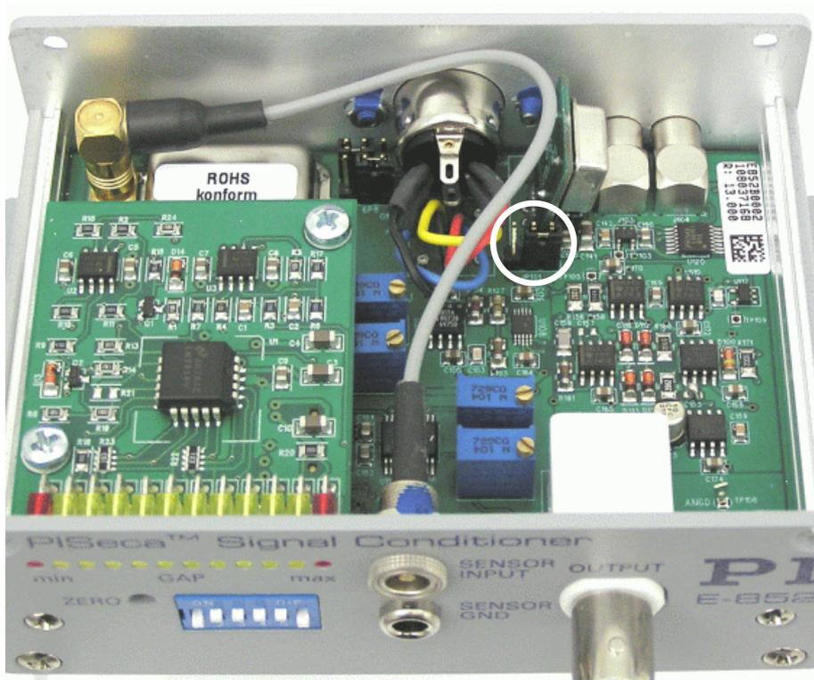
Fig. 12: E-852.10 with cover removed, jumper Jp 101 circled, set for internal generation of +5 VDC
