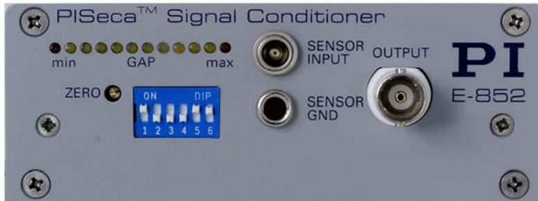
Fig. 4: E-852.10 front panel
