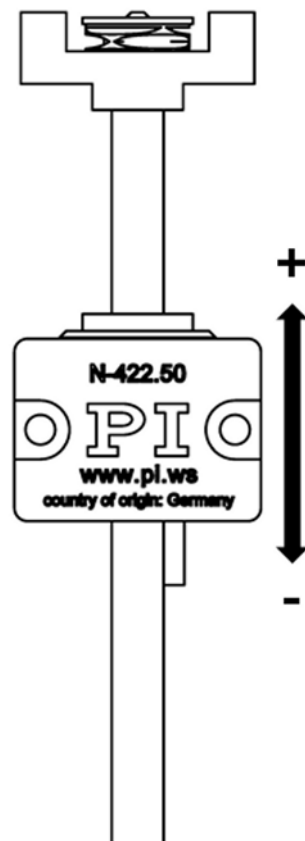
Figure 4: Directions of motion of the N-422
