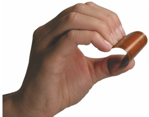
Fig. 3 Curvatures with radii as low as 20 mm are easily accommodated
