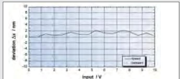
Fig. 4: Linearity of a P-752.11C, 15  $\mu\text{m}$  piezo nanopositioning stage operated with E-500/E-509.C1A control electronics. The travel range is 15  $\mu\text{m}$ , the gain 1.5  $\mu\text{m}/\text{V}$ . Linearity is better than 0.02%; even higher linearity is achievable with PI digital controllers
