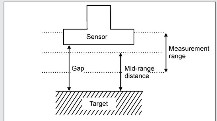
Fig. 14: Definitions: measurement range and mid-range distance have identical values
