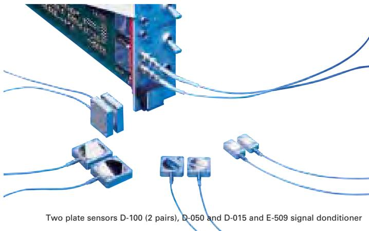
Two plate sensors D-100 (2 pairs), D-050 and D-015 and E-509 signal conditioner
