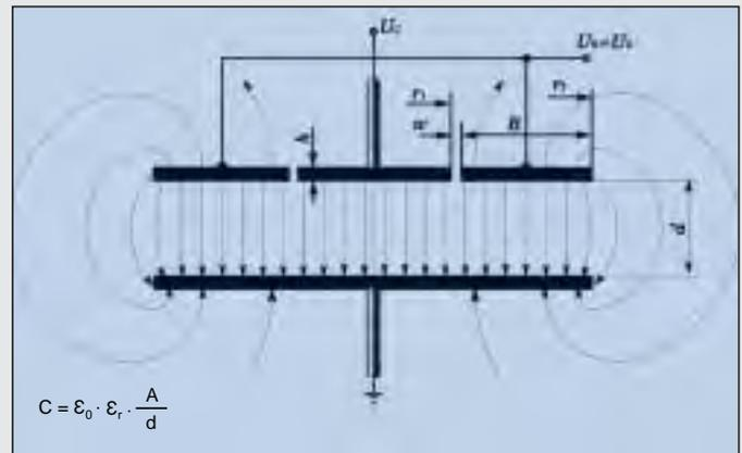
Fig. 6: Capacitive sensor working principle. The capacitance C is proportional to the active sensor area A,  $\epsilon_0$  is constant,  $\epsilon_r$  is the dielectric constant of the material between the plates, generally air
