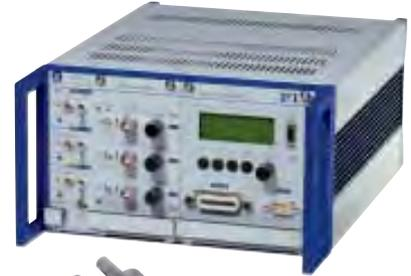
The E-509.E3 servo-controller module in an E-501 9.5" chassis with E-503 piezo amplifier module and E-516 PC-interface/display module provides servo-control of piezo nanopositioning systems with external PISeca™ D-510 capacitive 1-plate sensors (in front)
