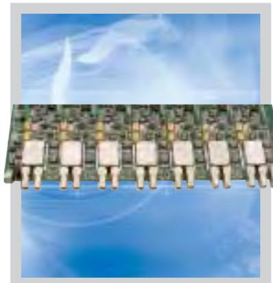
Custom, 7-channel, capacitive position sensor electronics
