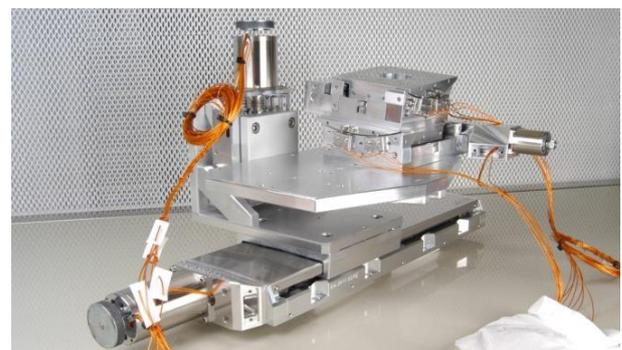
Fig. 2 Four axis system for ultrahigh vacuum application
