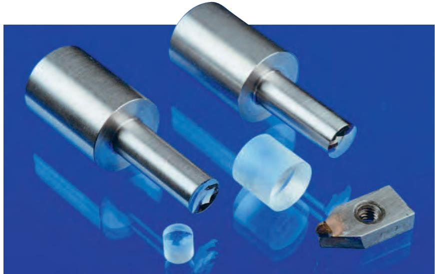
**Fig. 1:** The tighter the tolerances required for a product, the higher the precision required of the testing equipment. The optical mold inserts for production of plastic or glass lenses have especially high precision requirements. (Illustration: Fraunhofer Institute for Production Technology, IPT)
