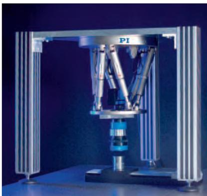
**Fig. 2:** The Hexapod is mounted on a 20 mm thick aluminum plate. The parallel-kinematic design and large aperture allow for the interferometer to be integrated into the Hexapod. Images are captured by a CCD camera and evaluated in real time. A MATLAB program, controls the position of the Hexapod. (Photo: Physik Instrumente, PI / Fraunhofer Institute for Production Technology, IPT)
