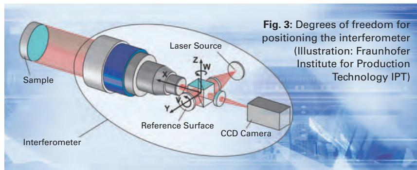
**Fig. 3:** Degrees of freedom for positioning the interferometer (Illustration: Fraunhofer Institute for Production Technology IPT)
