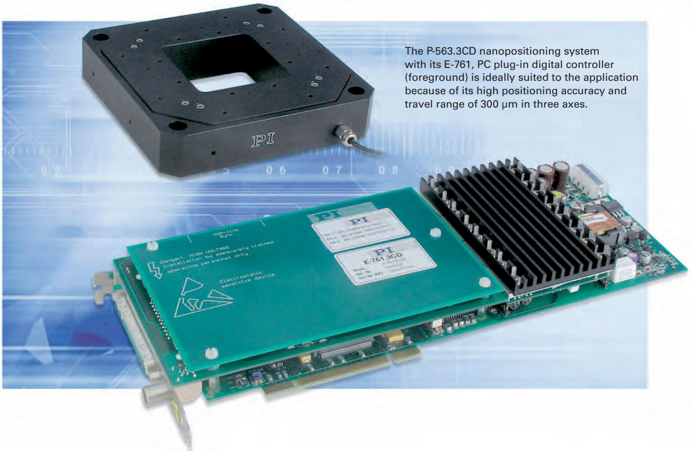
The P-563.3CD nanopositioning system with its E-761, PC plug-in digital controller (foreground) is ideally suited to the application because of its high positioning accuracy and travel range of 300 μm in three axes.
