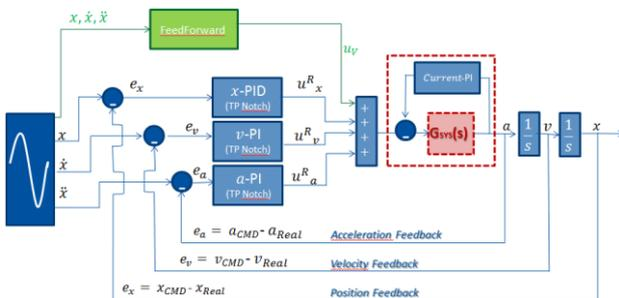
Figure 4. Control structure of a single hexapod leg that is decoupled from the other legs by design
