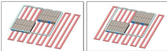
**FIGURE 6:** Tolerances on Halbach arrays have no influence on the forces generated at different X-Y positions. (Was already discussed in earlier paper by X.Lu et al.)
