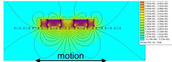
FIGURE 9: Flux simulation of one Halbach array
