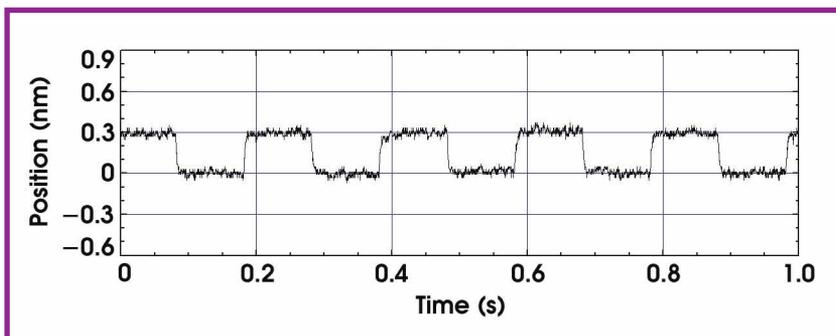
**Figure 5.** The 300-pm steps with the PicoCube show how fast and repeatably the system responds to positioning commands. The theoretical resolution (limited by electrical noise) is approximately 50 pm.
