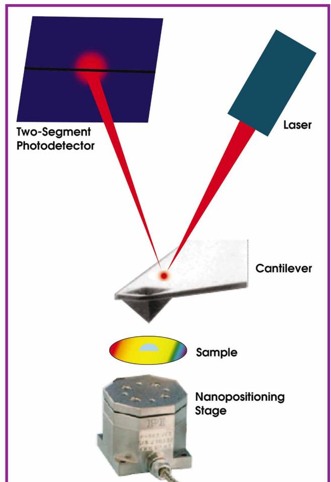
**Figure 1. The basic setup of the molecule stretching application involves the PicoCube stage moving the sample and measuring the position via an integrated subnanometre-precision capacitive sensor. The cantilever, laser and photodetector provide force feedback. Courtesy of Fernandez Lab.**
